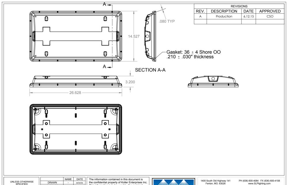
DIMENSIONS ARE IN INCHES TOLERANCES AS NOTED FRACTIONAL ±1/16" ANGULAR ±1° TWO PLACE DECIMAL ±.060 THREE PLACE DECIMAL ±.030
