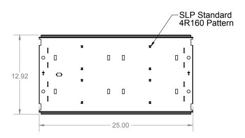
DIMENSIONS ARE IN INCHES TOLERANCES AS NOTED FRACTIONAL ±1/16" ANGULAR ±1° TWO PLACE DECIMAL ±.060 THREE PLACE DECIMAL ±.030
