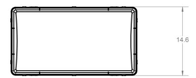
DIMENSIONS ARE IN INCHES TOLERANCES AS NOTED FRACTIONAL ±1/10" ANGULAR ±1° TWO PLACE DECIMAL ±.060 THREE PLACE DECIMAL ±.030
