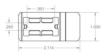
DIMENSIONS ARE IN INCHES TOLERANCES AS NOTED FRACTIONAL ±1/16" ANGULAR ±1° TWO PLACE DECIMAL ±.060 THREE PLACE DECIMAL ±.030
