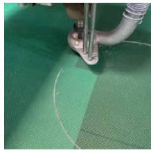
SLP Lighting has the capability to cut plastic or fiberglass material into precise shapes or create specific cutouts on our lighting products.
