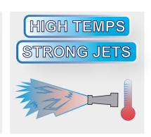
The IP Code, International Protection Code, sometimes also interpreted as Ingress Protection Rating, classifies and rates the degree of protection provided against the intrusion of dust, and water in electrical enclosures. IP69 means complete protection against contact dust and protection against the effects of high pressure and temperature water jets.
